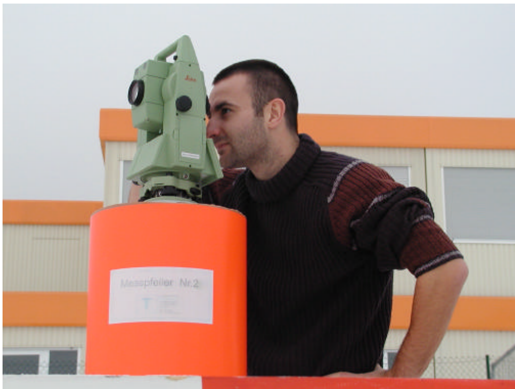
Fig. 1: Terrestrial measurements with the Leica TCRA 1103
