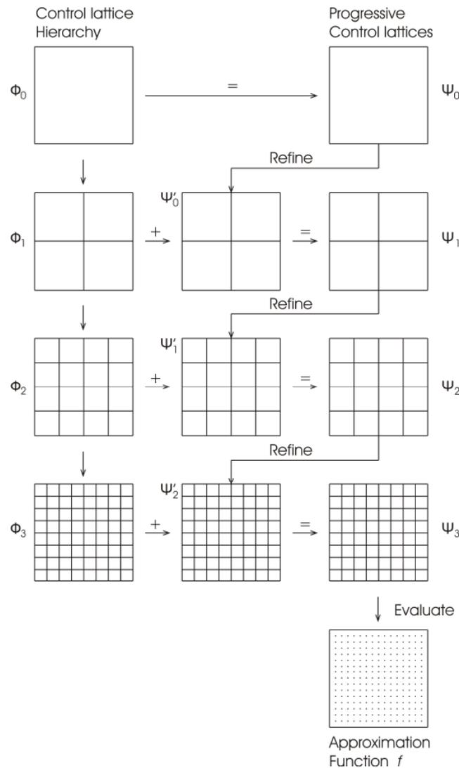
Figure 6: Approximation function evaluation in the MBA algorithm
