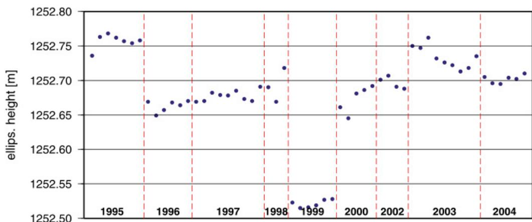
Figure 3: GPS station Fundata, daily solution for height coordinate for observations in campaigns between 1995 and 2004
