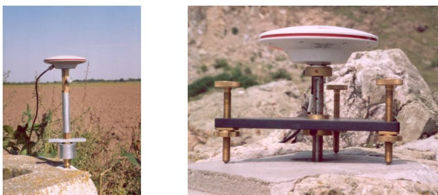
Figure 2: Different setups: CRC-adaptor (left) and triangular plate (right)
