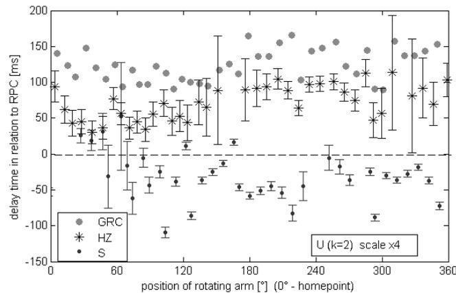
**Figure 8: kinematic measuring by a rotating velocity of 40°/s (horizontal rotating arm), GRC time, delay time for horizontal angle and distance. All times in relation to RPC. Measurement uncertainty scale x4**
